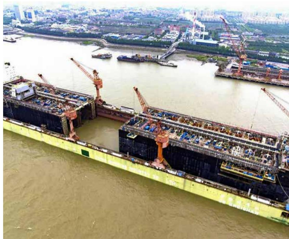
**Flashback: the mating of the P-70 FPSO hull at Cosco shipyard in an earlier phase of construction**
